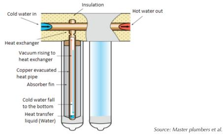
*Figure 4.3: Evacuated heat pipe*
