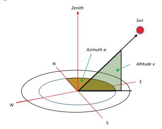
Figure 3.5: Altitude and azimuth angles.
