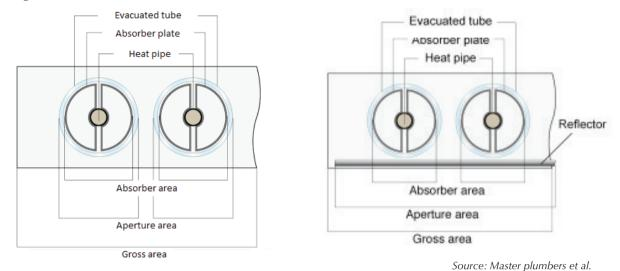
Figure 4.5: Cross-section of heat pipe with and without backing reflector.
