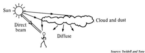
Figure 3.4: Direct and Diffuse radiation
