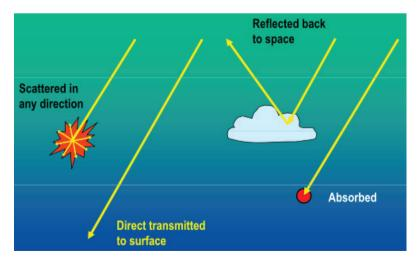
Figure 3.3: Illustration of how the solar radiation is reduced before reaching the earths surface.
