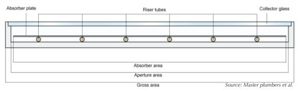
Figure 4.2: Cross-section of flat plate collector showing absorber, aperture and gross area
