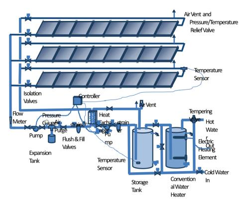
Fig 5.9: Parallel connected SWH system with vertical storage tanks (Andy Walker, 2013)
