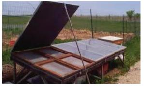
Figure 1.2: A locally made solar drier
