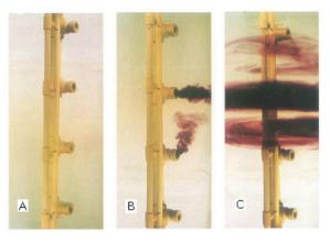
Figure 3.17: Using coloured water to show how stratification works. A) pipe with perforations in the tank; B) hot water comes out through different holes depending on its temperature; C) laminars of coloured water distribute themselves depending on temperature
