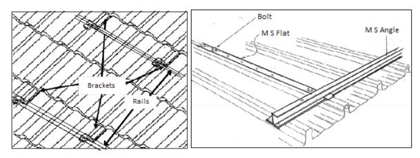
Figures 5.9: Example mounts on tile and box-type galvanized sheet
