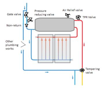
Figure 5.10: Direct passive system
