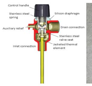
Figure 4.10: TPR valve schema and photo.
