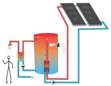
Figure 3.16: Active & indirect (closed loop) system
