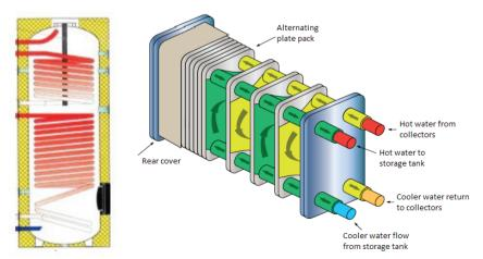
Figure 4.15: Schema of internal helical coils and external plate heat exchanger
