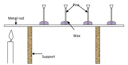
Figure 3.9: Heat transfer through conduction
