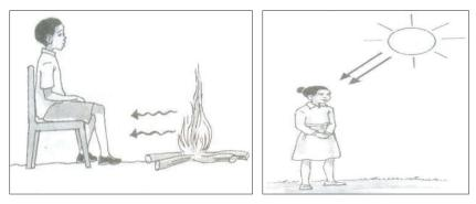
Figure 3.11: Radiation heat transfer from fire and the sun
