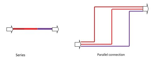
Figure 5.3: Illustration of parallel and series connection
