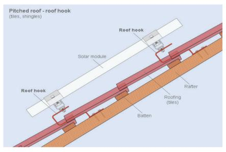
Figure 6.1: Standoff roof mounting structure on a tiled roof
