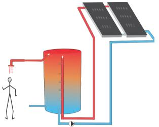
Figure 3.15: Active and direct system with stratification
