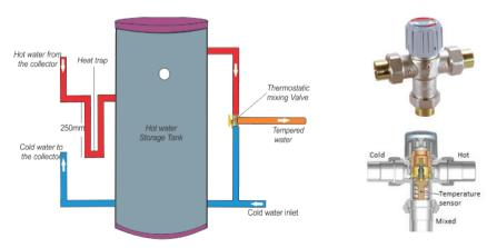
Figure 3.18: Schema of heat trap and thermostatic mixing valve
