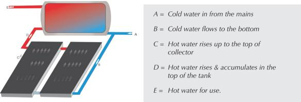
Figure 3.13: Illustration of a direct SWH system
