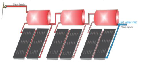
Note: All the piping in 20mm diameter It is recommended the installation of maximum five appliances
