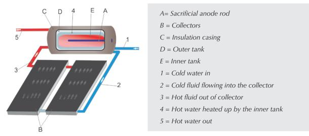
Figure 3.14: Illustration of an indirect SWH system
