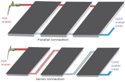
Figure 5.5: Parallel and series connected collectors
