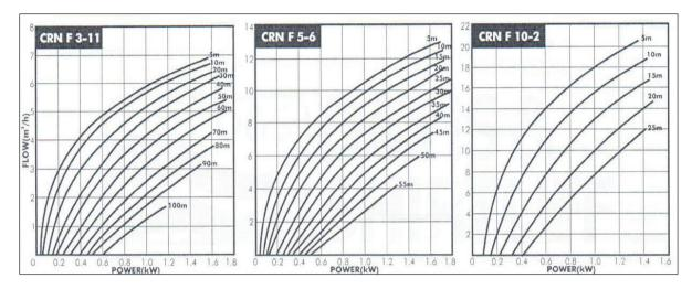
Figure 5.2: Pump Data Sheet
