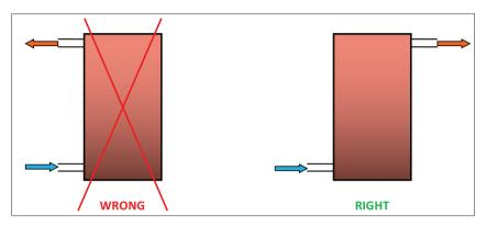
Figure 5.4: Balanced connection of collectors
