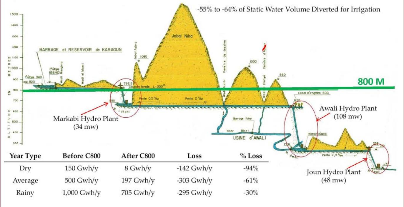
Figure 32. Impact of conveyors 800 M and 900 M on hydropower production. Schéma Directeur Hydro-Electrique au Liba, by Sogreah-Artelia, 2012, Beirut, Lebanon: Ministry of Energy and Water. Copyright 2012 by Ministry of Energy and Water.
