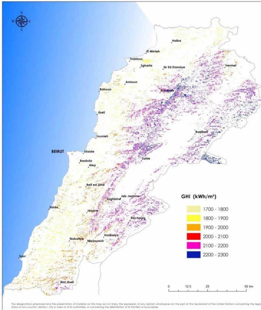
Figure 15. Filtered potential land areas for PV farms in Lebanon. (Source: [www.solar-med-atlas.com](http://www.solar-med-atlas.com))
