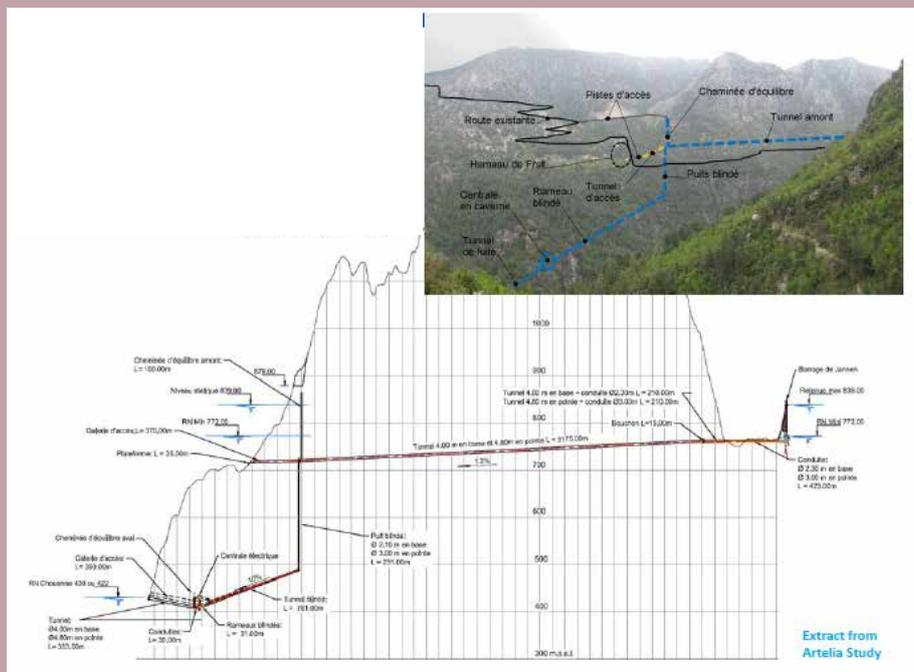
Figure 34. New dams Janneh hydroelectric plant. Reprinted from *Schéma Directeur Hydro-Electrique au Liban*, by Sogreah-Artelia, 2012, Beirut, Lebanon: Ministry of Energy and Water. Copyright 2012 by Ministry of Energy and Water.
