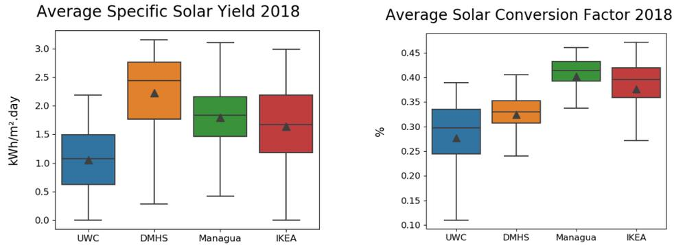
Fig. 12: Average specific solar yield (left) and average solar conversion factor (right) of each solar system in 2018. Median are displayed by a solid black line, quartiles are marked by colored boxes and the range of the measured data is displayed by the black whiskers. Averages are marked by black solid triangles.
