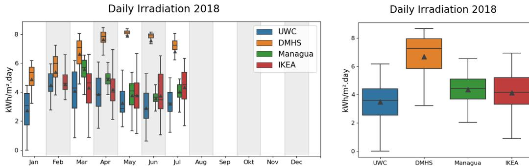
**Fig. 9: Daily average irradiation at each system in 2018. Black lines mark the median, the border of the colored boxes mark the quartile and the whiskers mark the range of the measured data. Averages are displayed as black triangles.**
