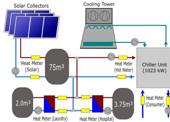
Fig. 5: Simplified hydraulic schema of MANAGUA.
