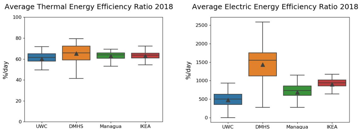
Fig. 13: Thermal (left) and Electrical Energy Efficiency Ratio (right) of each plant in 2018. Average values are displayed by black triangles, the median is displayed as horizontal line, the quartiles are marked by the coloured boxes and the range of the calculated data is marked by the black whiskers.
