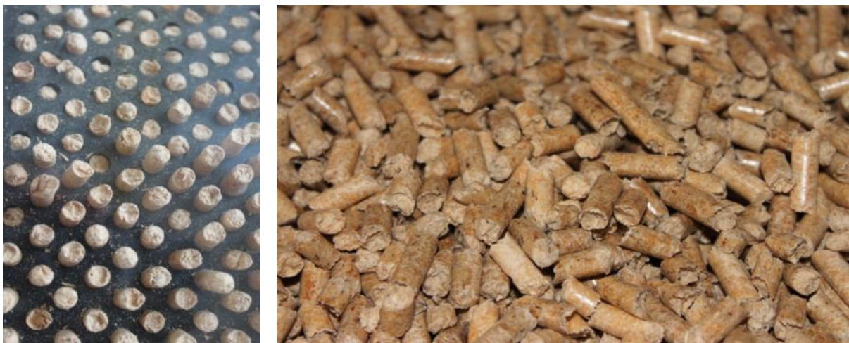
Figure 13: Pellet press (left) and high-quality pellets (right) (Source: Rutz D.)
