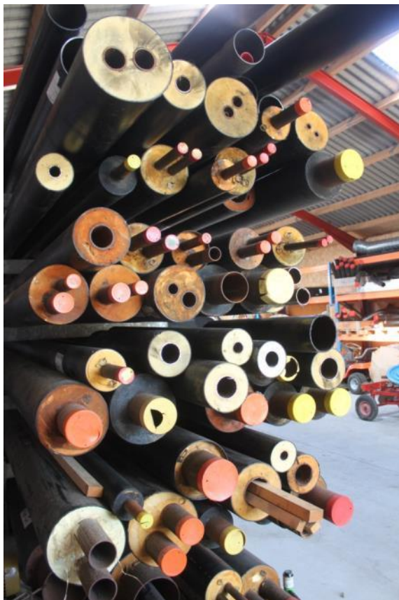
Figure 50: Samples of old single and double steel pipes (left) and double polymer heat pipe (right) (Source: Rutz D.)
