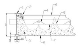
Figure 29: Photo of CPC AO SOL solar collector.
