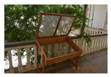
Figure 20: Fruit dehydrator used by a NGO in S. Vicente to dry fruits (experimental) – photo taken at Mindelo International School of Arts
