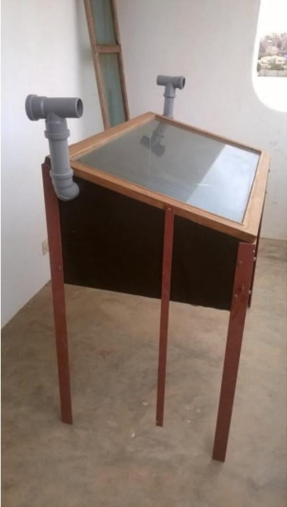
Figure 21: Solar dryer for home use (fruit drying) – photo provided by owner of dryer (Ms. M.M. Estrela)
