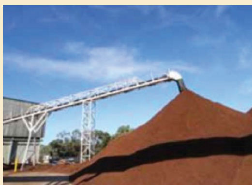
Automatic feed handling and 8MW th boiler using grape marc, photos Australian Tartaric Products
