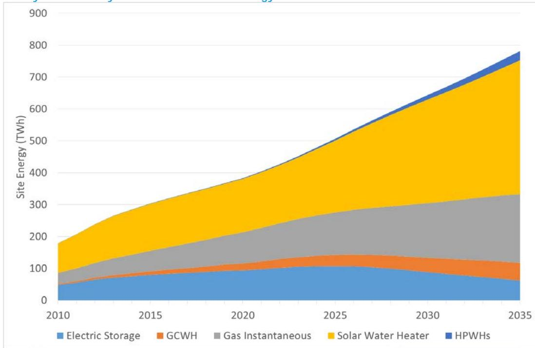
Figure 22. Estimated Water Heater Final Energy Consumption in China for the Least Life Cycle Cost Scenario by Water Heater Technology
