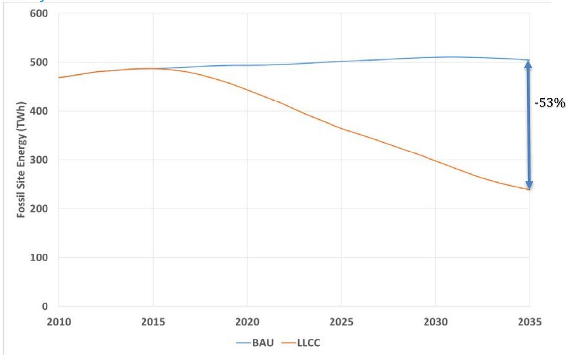
Figure 35. Estimated Water Heater Primary Energy Consumption in the US for the BAU and Least Life Cycle Cost Scenarios
