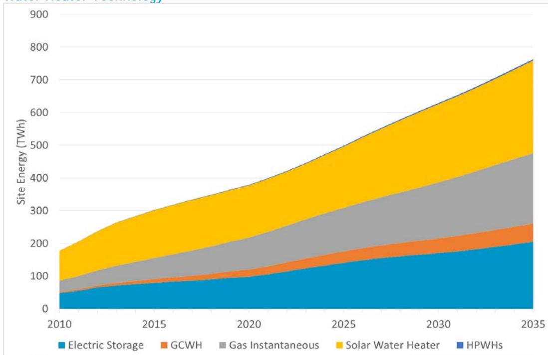
Figure 21. Estimated Water Heater Final Energy Consumption in China for the Recommended Policy Scenario by Water Heater Technology
