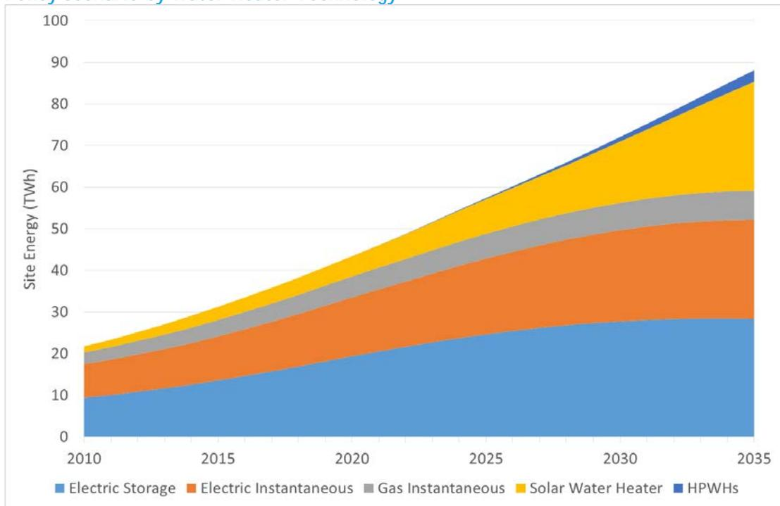
Figure 32. Estimated Water Heater Final Energy Consumption in India for the Least Life Cycle Cost Scenario by Water Heater Technology
