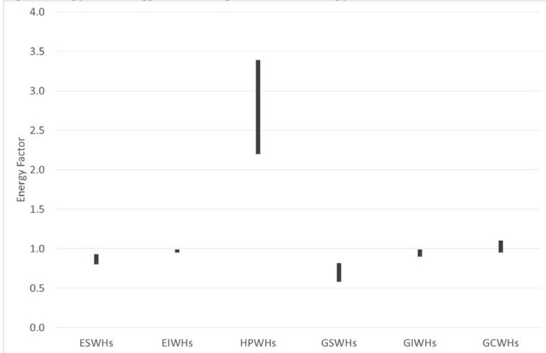
Figure 2. Typical Energy Factor ranges for different types of water heater after adjusting for primary to secondary energy losses
