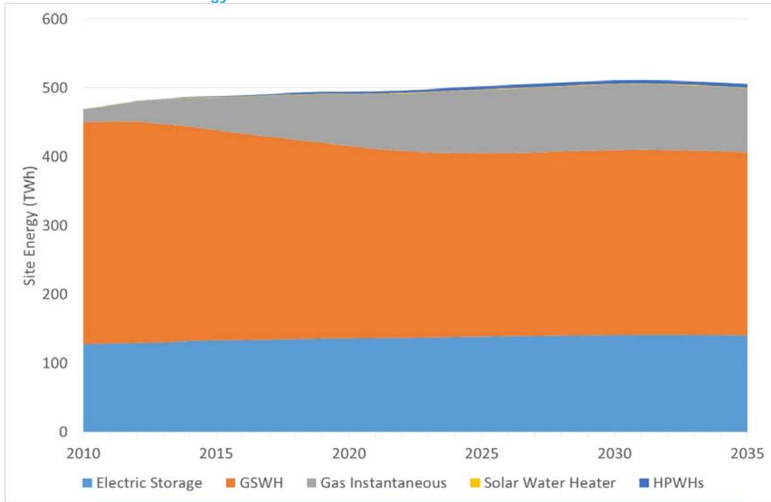
Figure 41. Estimated Water Heater Final Energy Consumption in the US for the Recommended Policy Scenario by Water Heater Technology
