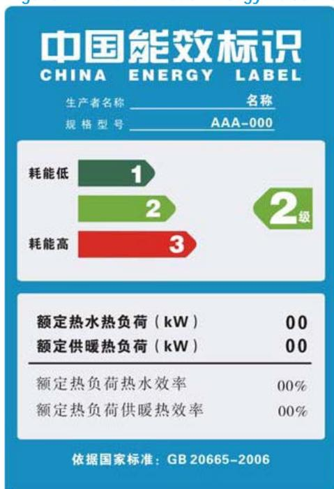
Electric storage water heaters are divided into five grades of energy efficiency, of which Grade 1 represents the highest energy efficiency. The required standing loss per 24 h and hot water output rate for each grade of electric water heater are shown in Table 2.7.
