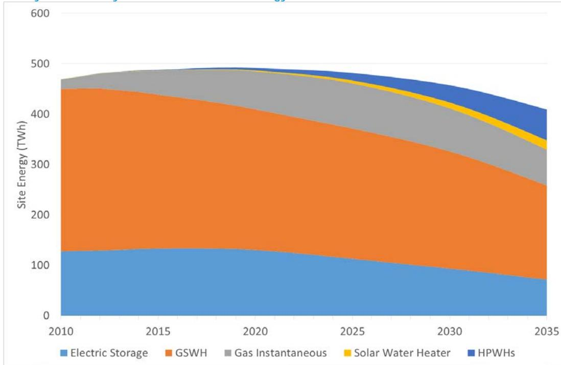
Figure 42. Estimated Water Heater Final Energy Consumption in the US for the Least Life Cycle Cost Scenario by Water Heater Technology
