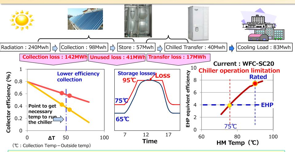
Collection operation is limited in the low efficiency side due to the Chiller's operation start temp(85℃) and Stop Temp (75 ℃).
