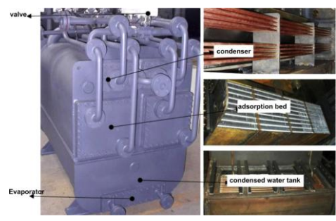
Fig. 6 Silica gel-water adsorption chiller.
