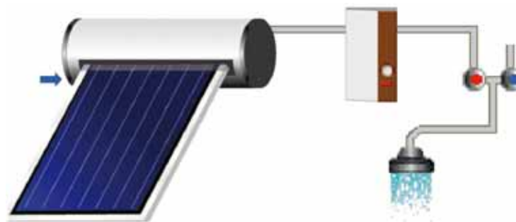
Figure 46: Hydraulic scheme of the domestic hot water thermosiphon reference system for single family houses
