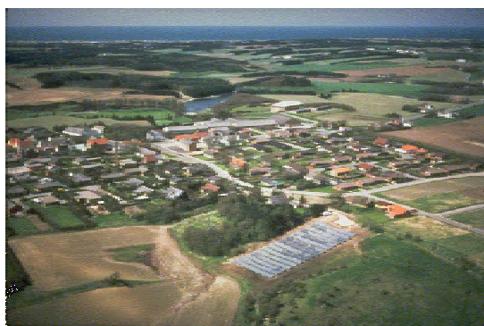
1000 m 2 collector array in Saltum.
