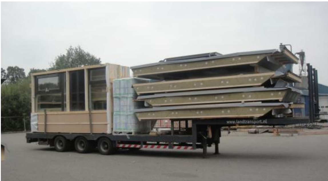
Figure 13: One truck load=one house ready for transportation at the factory
