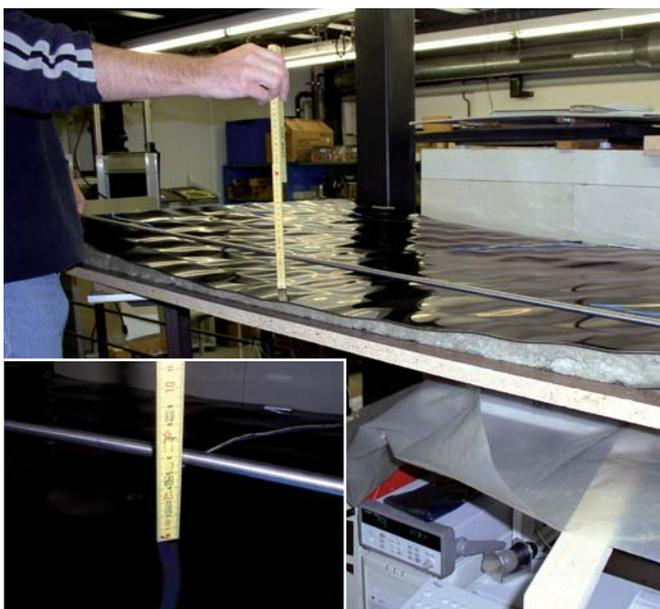
Figures 10 & 11: Significant dished deformation led to an overall curvature with a depth in the range of 5 - 6 cm.
