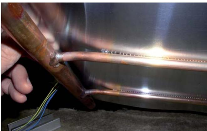
Figure 14: Mild separation of one of the ascending pipes.
