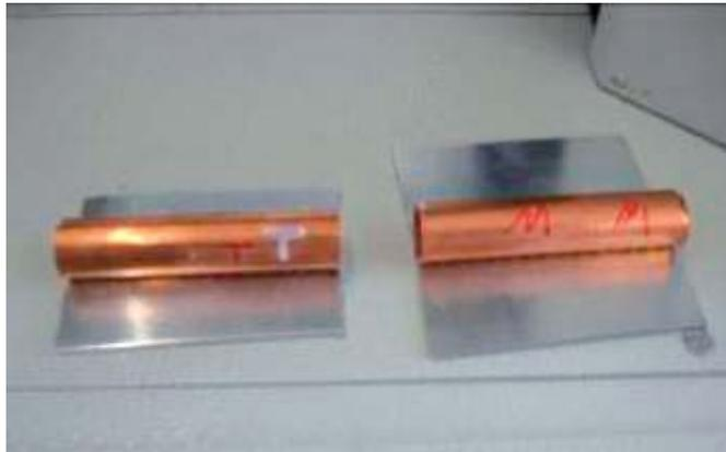
Photograph 2: Welding sample – before test
