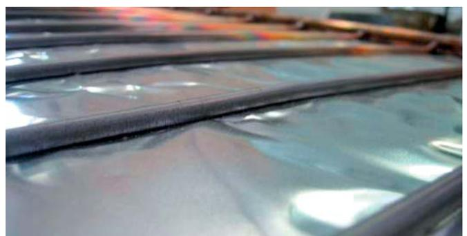
Images 3 and 4: Close-up photos showing the ripples on the absorber plate.
