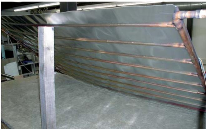
Figure 13: Backside of absorber following 1000th cycle.
