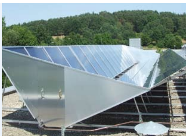
Fig. 2: Field with prototypes of improved flat-plate collectors (under construction). The collectors are double covered (solar glass and plastic foil) and equipped with external reflectors.
