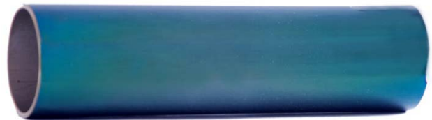
Sputter deposited TiAlN/TiAlON solar selective coating on 6" stainless steel tube
