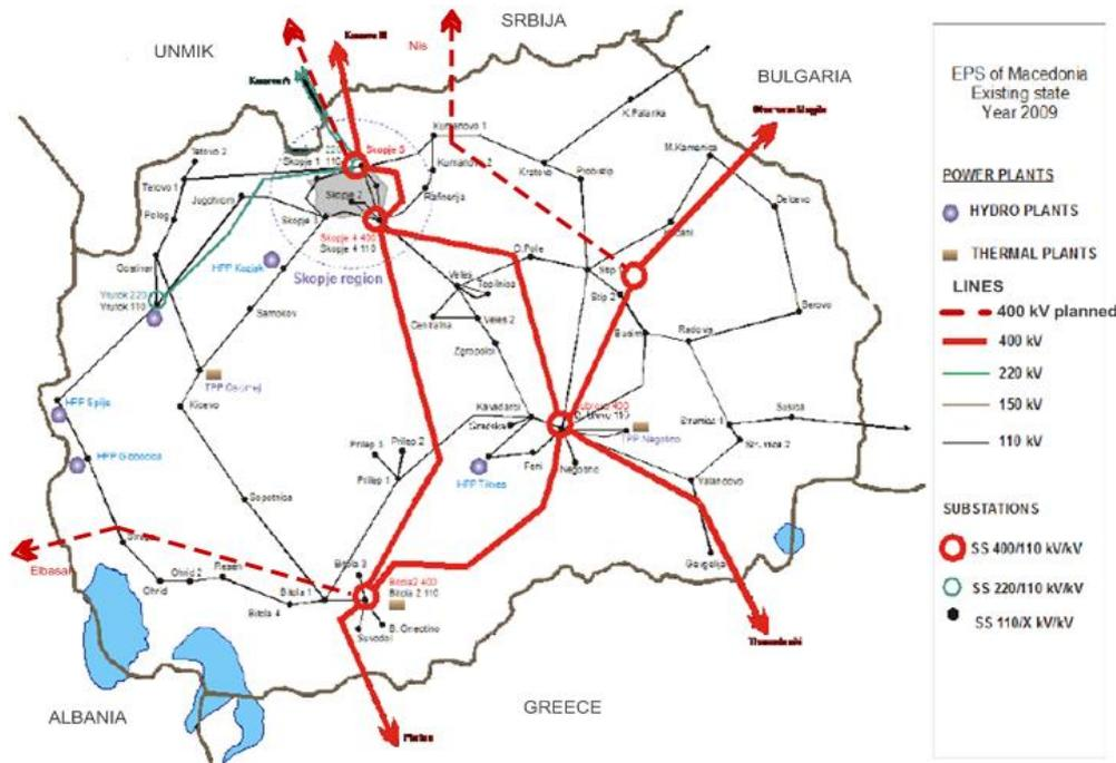
Figure 3.2.2.1. Existing and planned structures of the transmission system of the Republic of Macedonia
