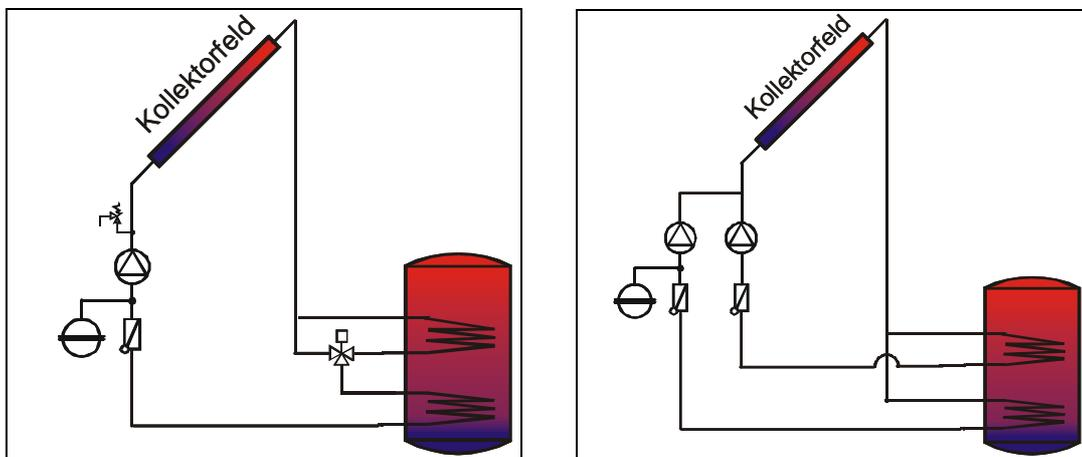
Figure 11: Examples of immersed heat exchanger at two levels; left: one or BOTH heat exchanger are used; right: one OR the other heat exchanger is used
