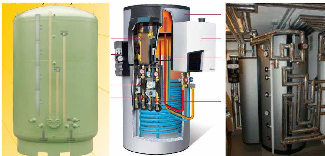
Figure 74: Examples of tank designs with pipe connection at tank side in medium/low temperature zones with internal pipes to the top; Source: Pink (left) Bösch (middle); example of well insulated piping and thermosiphon heat traps at all pipe connections at the heat storage (right; Source: Tisun)
