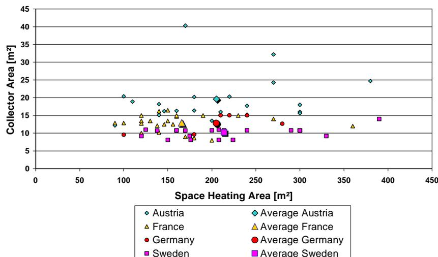
Figure 22: Space heating Area and Collector Area of the evaluated houses.
