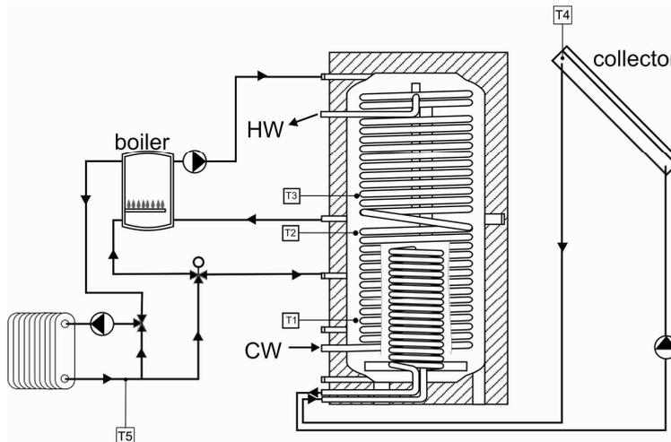
Figure 69: System design of the solar combisystem 1
