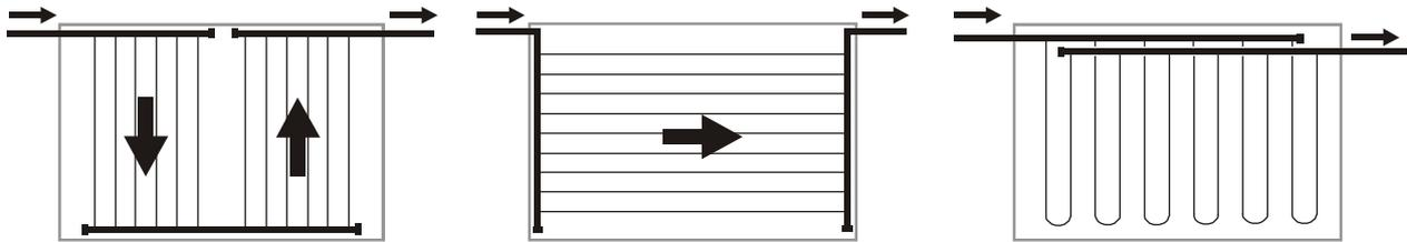
Figure 83: Collectors with bad emptying behaviour
