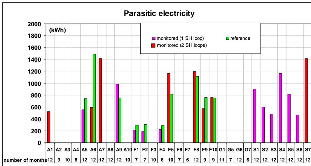
Figure 64: Parasitic electricity consumed
