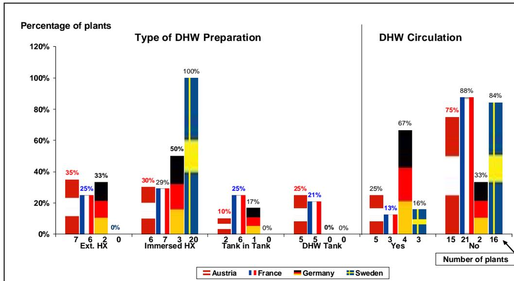
Figure 49: Type of domestic hot water preparation
