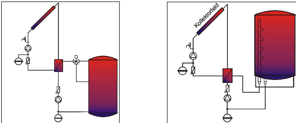
Figure 12: External heat exchanger with: left: two pipe connections at two different level (external stratification via switching valve); right: internal stratification device
