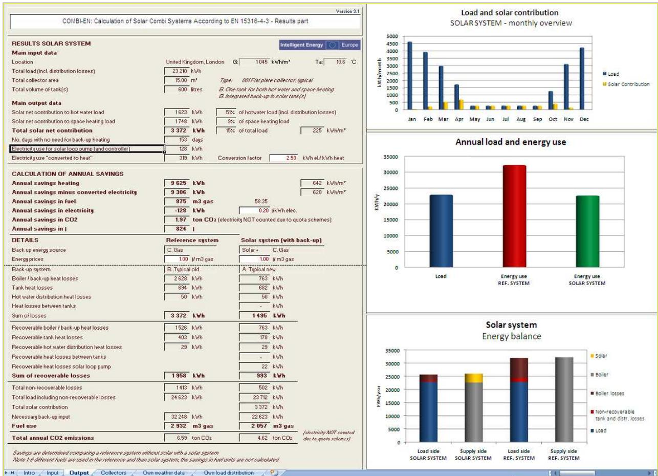
Figure 86: COMBI-EN result sheet - example
