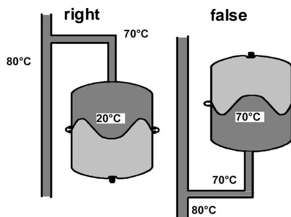
Figure 80: Right and false way for connecting an expansion vessel in a solar thermal system (left).
