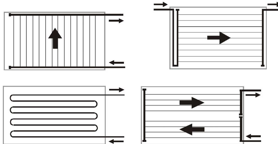
Figure 84: Collectors with good emptying behaviour
