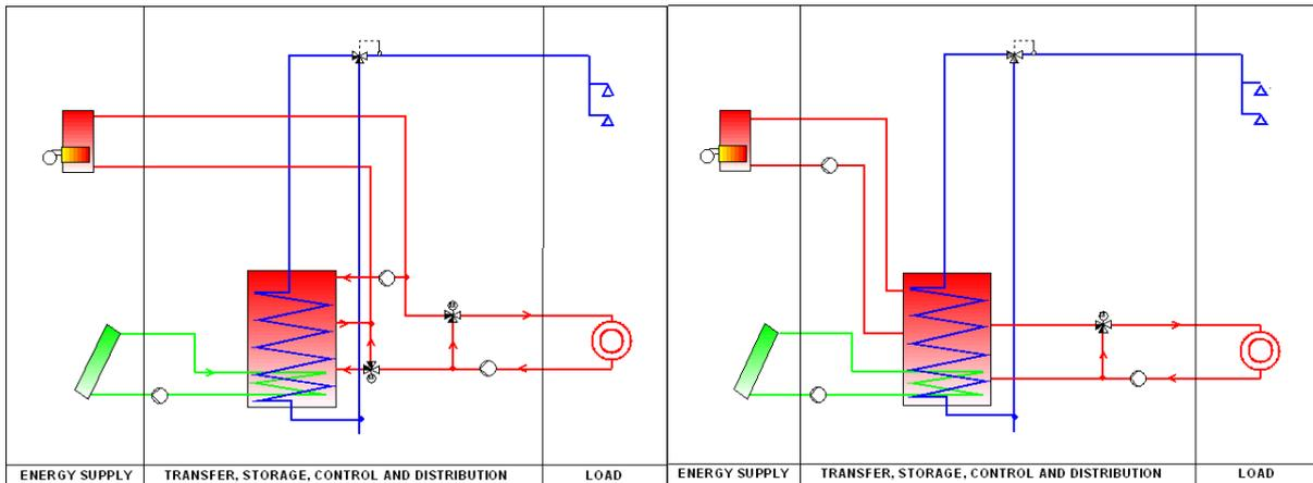
Figure 8: Hydraulic scheme of a heat storage system with an immersed heat exchanger – auxiliary boiler is integrated as return flow increase (left) or is charging the heat storage tank (right)
