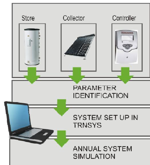
Figure 68: Principal structure of the CTSS-method
