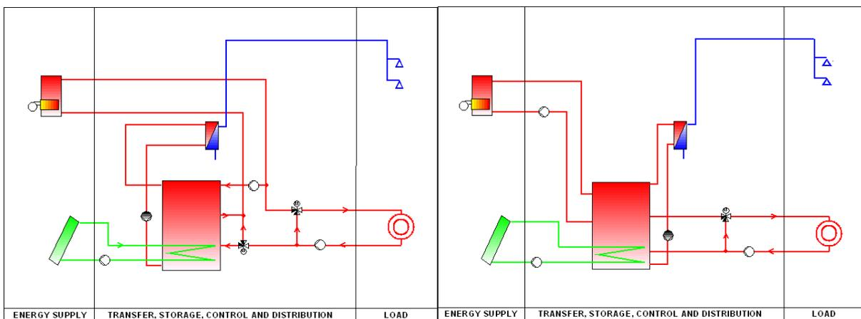
Figure 9: Solar heating plant with a fresh water unit – auxiliary boiler is integrated as return flow increase (left) or is charging the heat storage tank (right)
