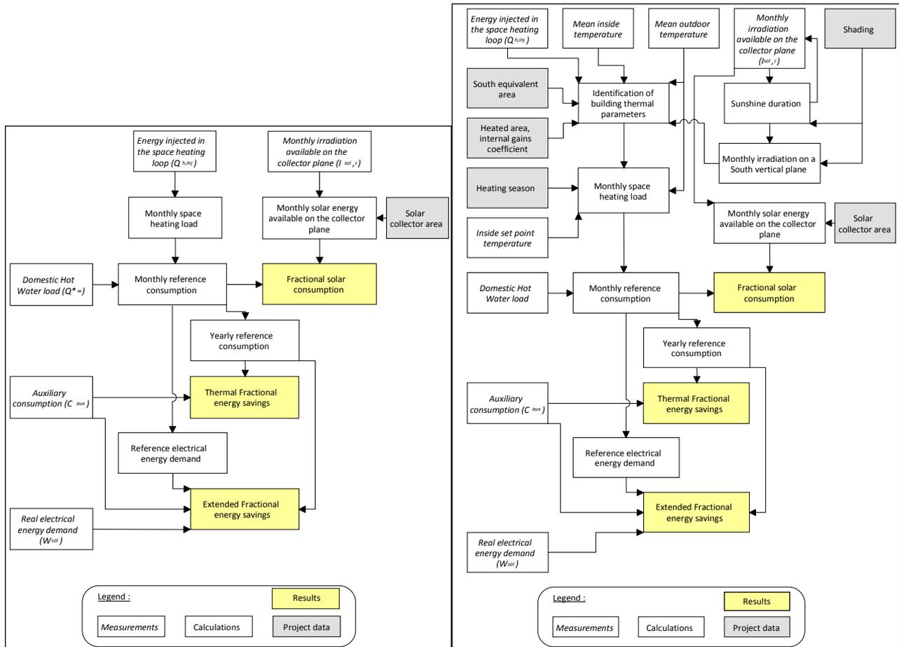
Figure 54: Monitoring diagram for systems without (left) and with (right) storage for space heating in the building
