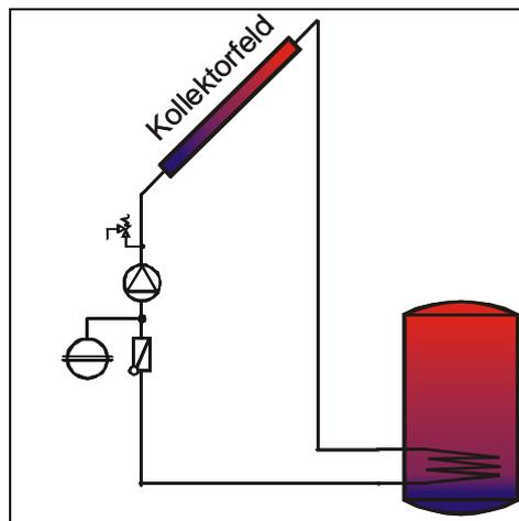
Figure 10: Immersed/internal heat exchanger at one level
