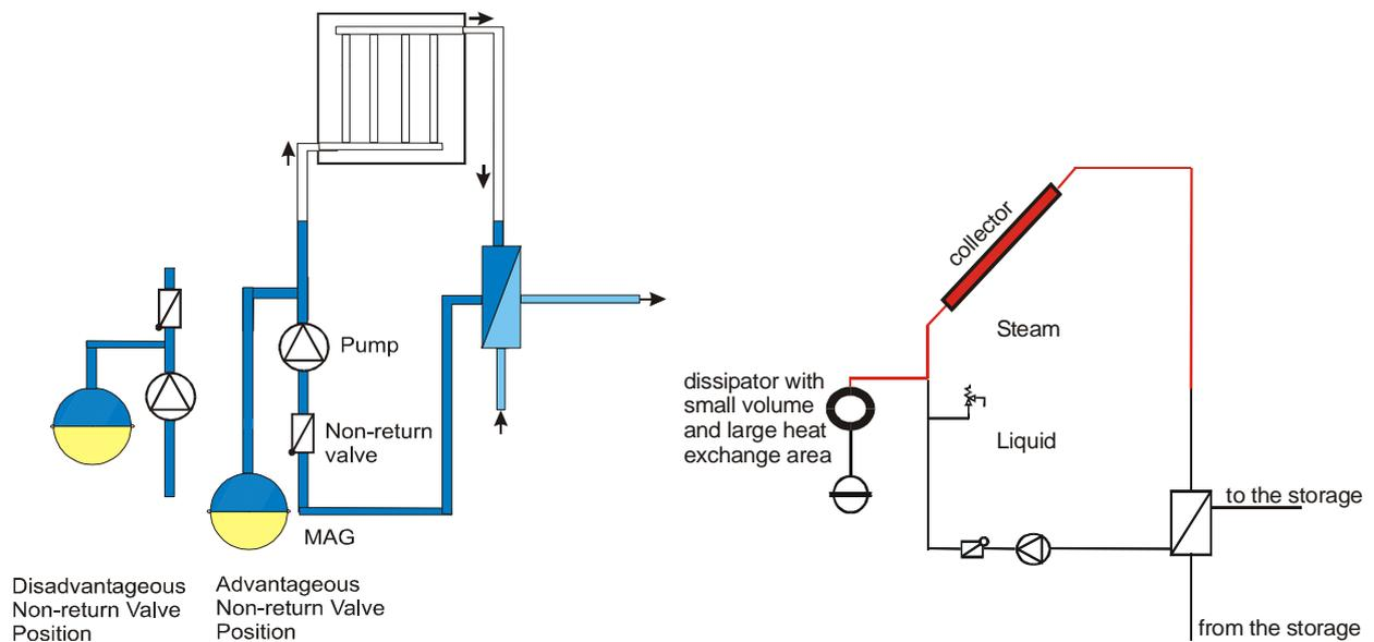
Figure 82: Correct position of the non-return valve in relation to the expansion vessel (left) and correct position of a stagnation cooler keeping the steam above temperature critical components (right) (Source: AEE INTEC)
