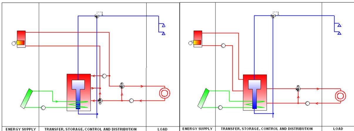
Figure 7: Hydraulic scheme of a tank-in-tank system – auxiliary boiler is integrated as return flow increase (left) or is charging the heat storage tank (right)
