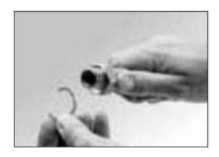
Slide on 1" union nut and close segment ring around pipe groove.
