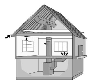
Fig. 3: Ductwork in house with ASR roofing tile
