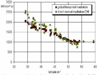
Figure 2: Solar irradiation Vs latitudinal position [12].
