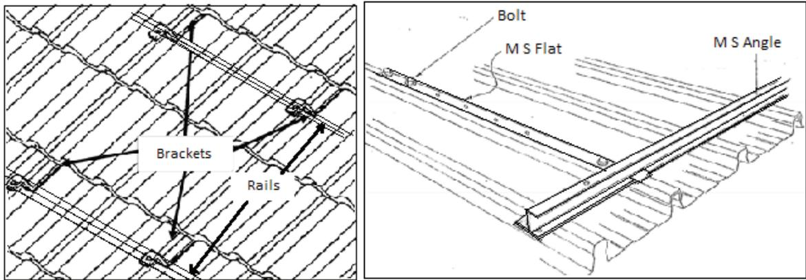
Figures 5.9: Example mounts on tile and box-type galvanized sheet
