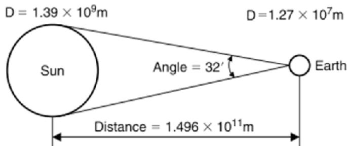
Figure 3.2.: Distance between the sun and earth (D= diameter).
