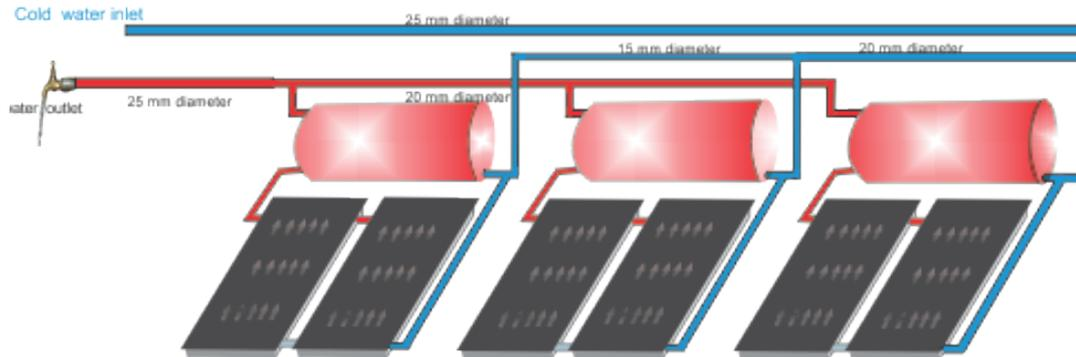
Figure 5.6: Parallel connection of multiple systems
