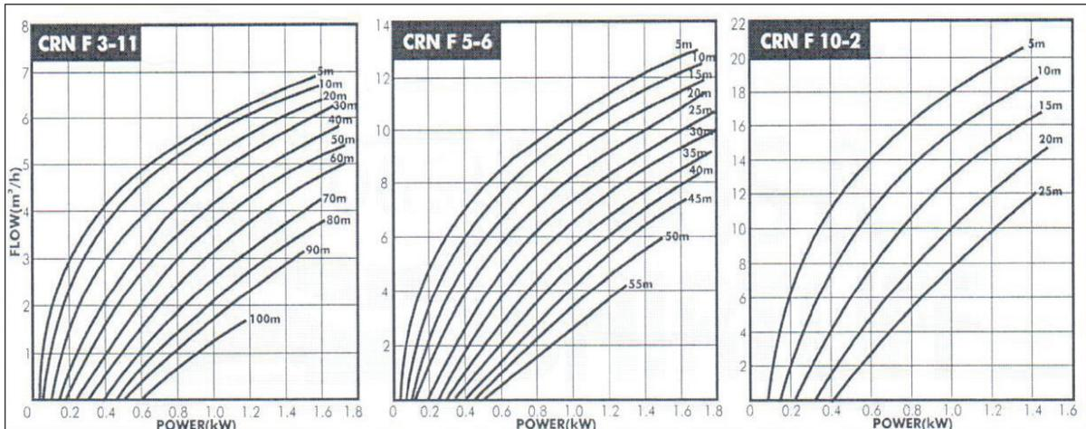
Figure 5.2: Pump Data Sheet
