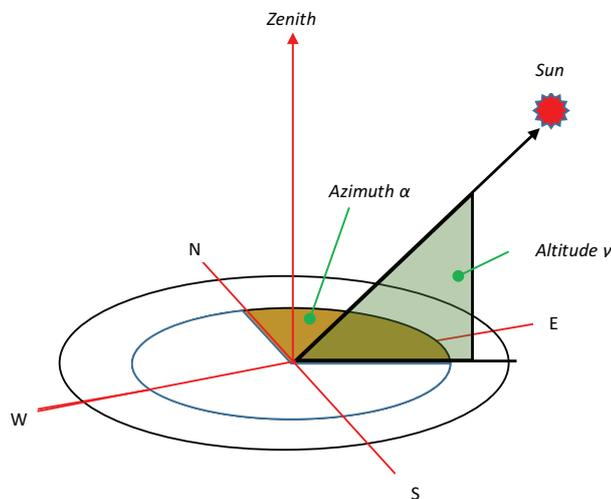
Figure 3.5: Altitude and azimuth angles.
