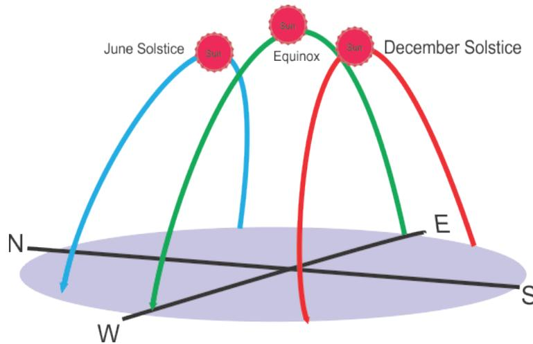
Figure 3.6: Typical 3-D appearance of Sun Path in Kenya.
