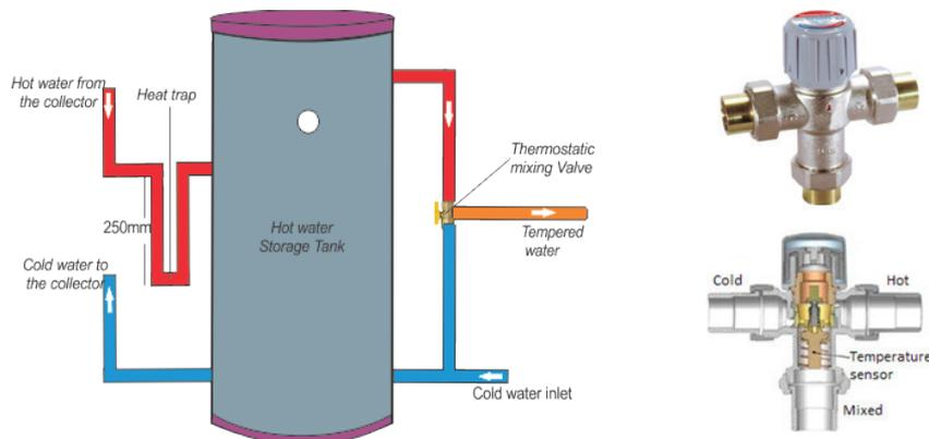
Figure 3.18: Schema of heat trap and thermostatic mixing valve
