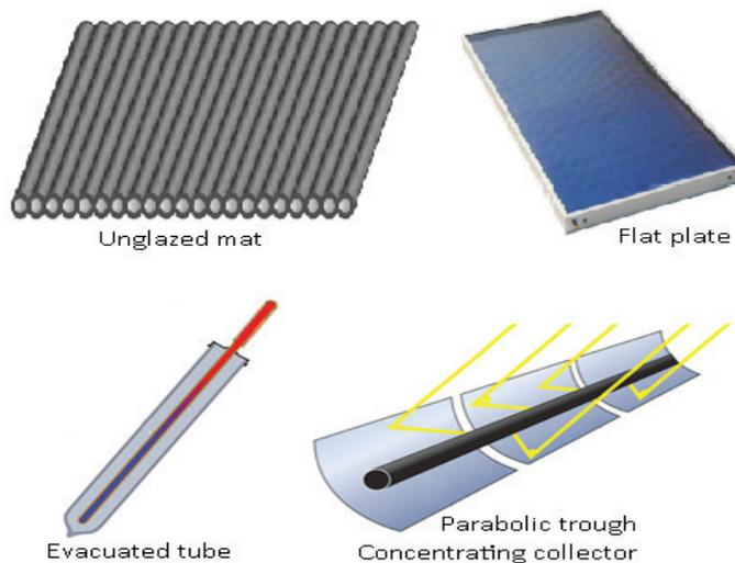
Figure 3.12: Example of collectors for various applications
