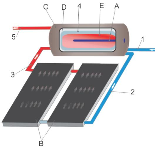
Figure 3.14: Illustration of an indirect SWH system
