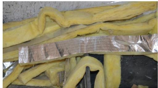
Figure 4.14: Fibre glass linings with aluminium foiling – by steelstone
