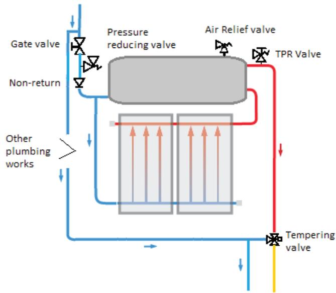
Figure 5.10: Direct passive system
