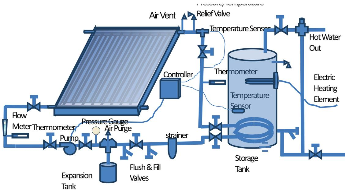
Figure 4.19: Use of a controller and other components in a closed loop, active SWH system (Andy Walker, 2013)
