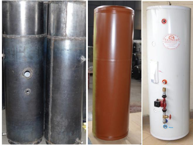
Figure 4.8: Tanks after fabrication, spray painting of jacket and complete tank – by Steelstone
