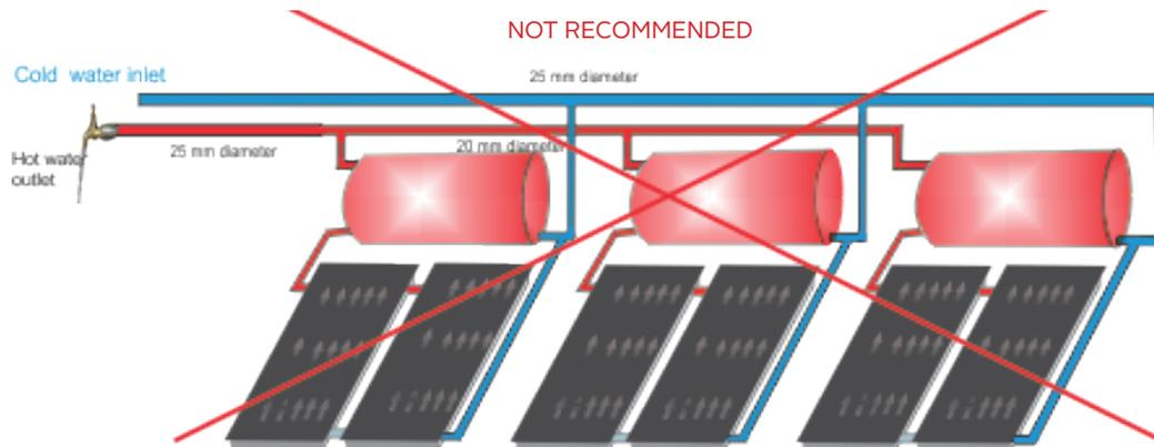
Figure 5.7: Imbalanced parallel connection of multiple systems
