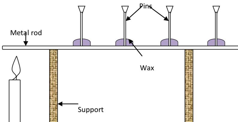
Figure 3.9: Heat transfer through conduction
