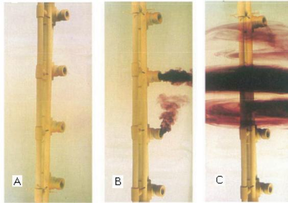
Figure 3.17: Using coloured water to show how stratification works. A) pipe with perforations in the tank; B) hot water comes out through different holes depending on its temperature; C) laminars of coloured water distribute themselves depending on temperature
