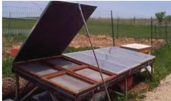
Figure 1.2: A locally made solar drier
