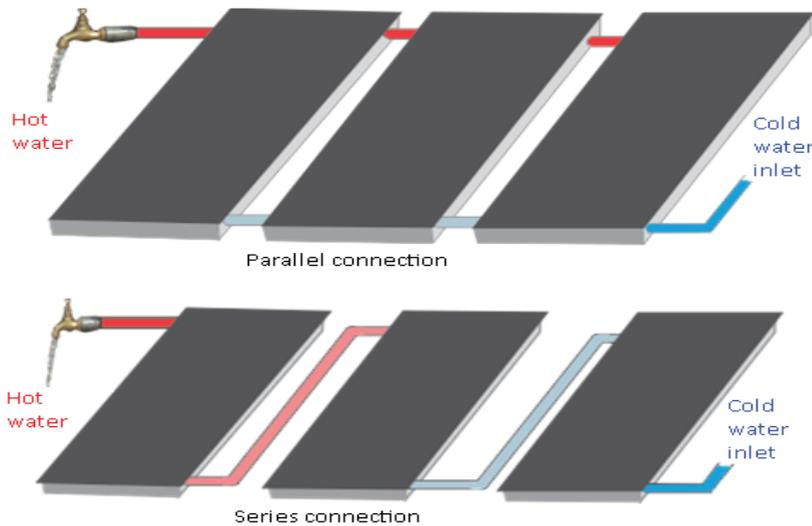
Figure 5.5: Parallel and series connected collectors
