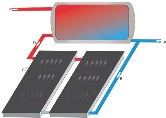
Figure 3.13: Illustration of a direct SWH system
