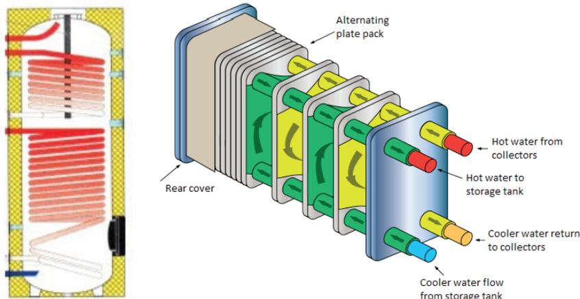
Figure 4.15: Schema of internal helical coils and external plate heat exchanger
