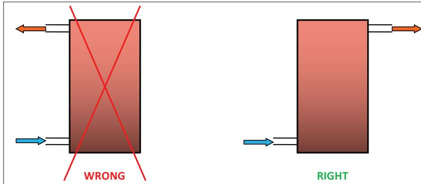
Figure 5.4: Balanced connection of collectors
