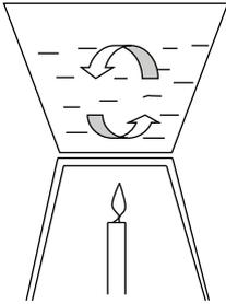
Figure 3.10: Convection heat transfer in liquids
