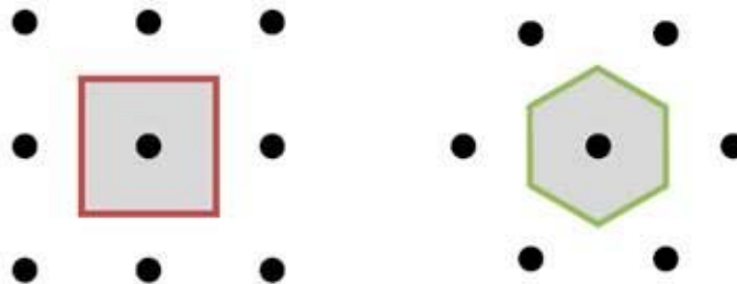
Figure 3.3 Top view of borehole section areas of 7.76 m 2 for a square pattern and a “honeycomb” pattern (from 86 )
