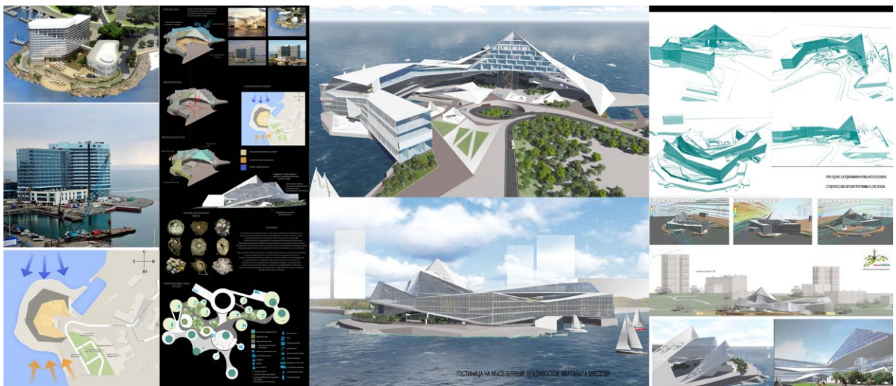
Fig. 13. The new buildings in Vladivostok gives a unique material for the study of the microclimate. The study of the microclimate of the new hotel on Cape Burnyi allowed Margarita Shvedova to develop an alternative form of the building. Closed from the wind and open to the sun courtyard creates a comfortable environment for citizens. While the realized tower forms flows of the strong wind on it’s territory.
