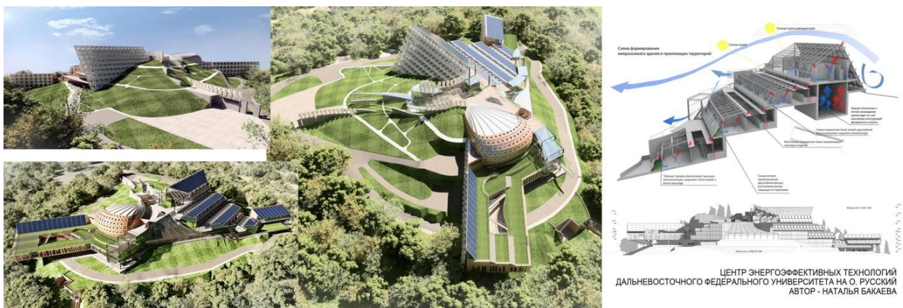
Fig. 23. Graduation Project, Bachelor's Program. "Research Center of Energy Efficient Technologies for FEFU". Motto: open the "building face" to the sun, oppose "back" to the wind, and from the north - push the building into the landform. FEFU campus buildings (phase I) on Russky Island facing north fully glazed facades, and the streets of the western part of the campus create solid wind corridors, since they are stretched along the prevailing direction of the monsoon. Partial presentation. Author - Natalia Bakaeva.
