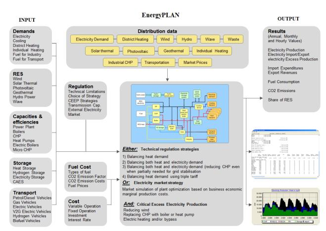
Figure 12: The structure of the EnergyPLAN tool [17].
