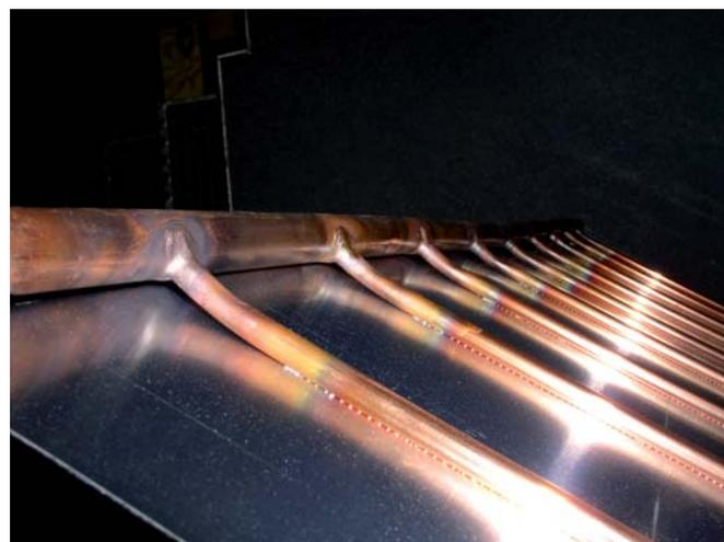
Figure 7: Rear side of absorber.
