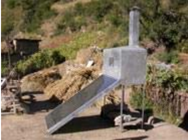
A community solar drier Solar drier drying cabinet with 6 drying trays
