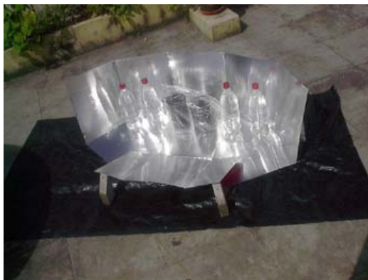
3-Plated Solar Panel Cooker Pasteurizes one Liter water in 01 hr.
