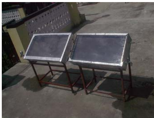
Solar Water Pasteurizer Pasteurizes 14-16 liters water in a day and keeps hot for 10-12 hours after sunset.
