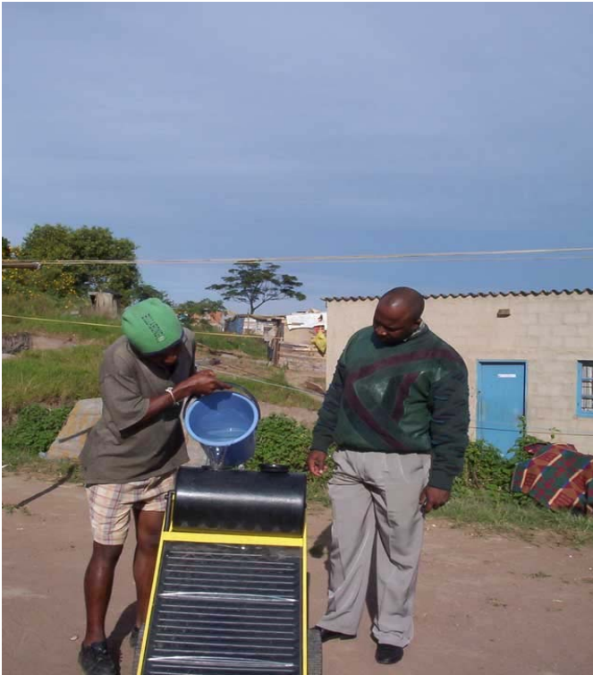
Figure 8: Filling a portable solar water heater with water. Photograph: Solar Engineering Services
